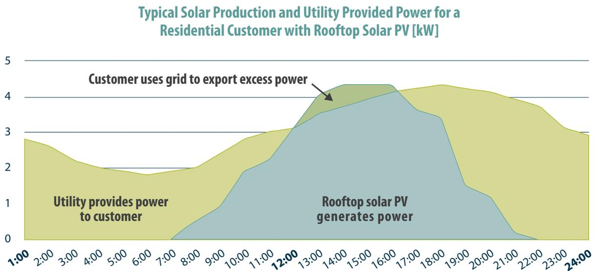
Figure 2 Solar production example with customer exporting energy back to the grid.
